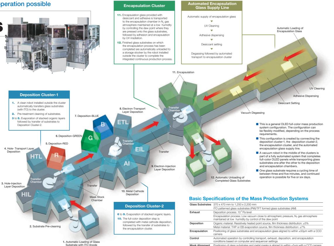
Mask Alignment Positioning of glass substrates and metal masks is aligned to within ±5µm with a CCD camera
